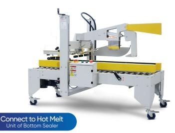
Add Hot Melt System The Hotmelt System of Carton Erector can also feed the Top Sealer by adding: 1 Hose, 1 Applicator, 2 Modules and 4 Nozzles
